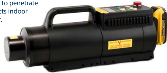
Exposure through 141 mm solid concrete curb with High Energy by Evo source
